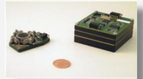
>> CSA96 COMPACT LARGE POWER SWITCHING AMPLIFIER FOR LINEAR MAGNETIC ACTUATOR
